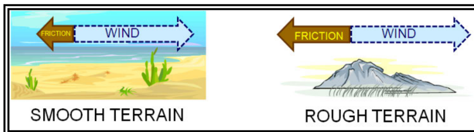
Figure 7-6. Friction Force Magnitude Variations with Terrain Roughness
