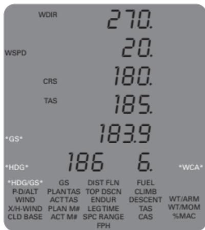
**Note:** Wind direction and direction of flight must be entered consistently relative to true or magnetic north for accurate calculations.
