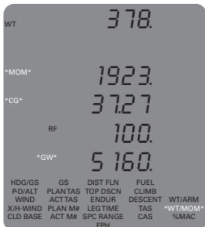
Totals for moment, center of gravity, and gross weight should then be checked against the aircraft's approved operating limits.
