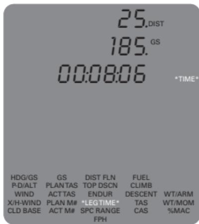
After **LEG TIME** is calculated, the count down timer can be activated starting at the calculated time by pressing
