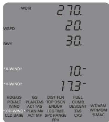
**Note:** Wind direction and direction of flight must be entered consistently relative to true or magnetic north for accurate calculations. Right crosswinds are shown as positive numbers, while left crosswinds are shown as negative numbers. A positive value for **H-WIND** denotes a tailwind, while a negative value denotes a headwind.
