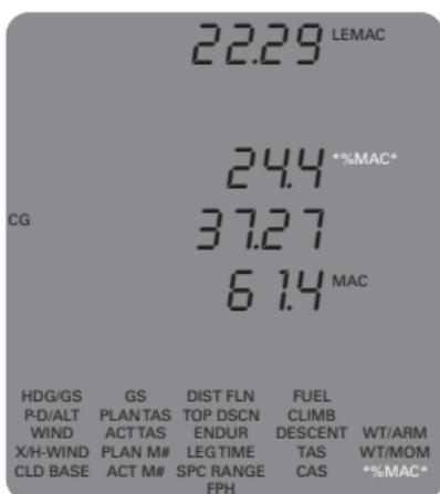
The total for **%MAC** should be checked against the aircraft's approved operating limits.
