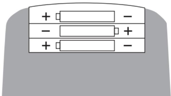
1. Batteries should last from six to nine months depending on use. If your E6B fails to respond or the display becomes dim, replace the batteries. Installation of new batteries should be checked to ensure proper placement.
