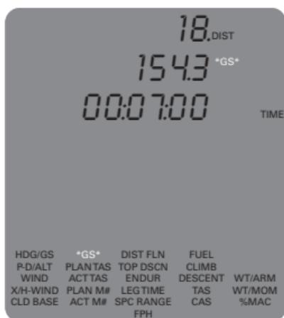
**Note:** Times can be imported from the timer for ground speed calculations. This can be done by pressing **TIMER** **ENTER** when the computer prompts for TIME to use the timer's current value.
