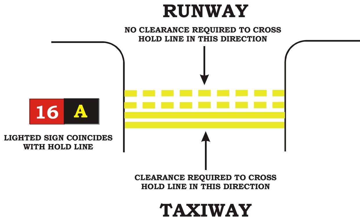
All aircraft on the runway side of the hold line are under the authority of the tower controller. Before crossing the hold line onto the active runway, pilots of taxiing aircraft must receive a clearance to do so from the tower controller.
