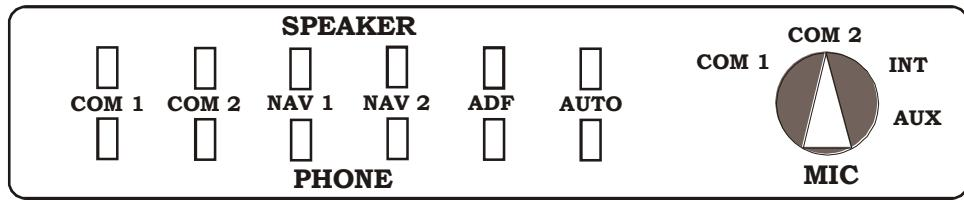
Transmitter selection is controlled by the MIC switch on the right. Reception is controlled by the buttons (or switches) to the left. The top row of buttons (or switch positions) direct audio output to the cabin speaker, while the bottom positions direct output to the headphone jacks.
