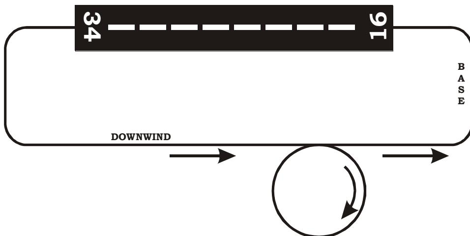
Two-seventy: Execute a 270-degree turn at the end of the downwind leg, and re-enter the traffic pattern on base to provide for traffic spacing.
